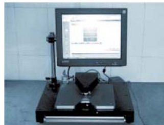
MS203 wafer tester (Resitivity, thickness ,TTV)
