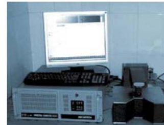
Life time tester (SEMILAB WT-1000)
