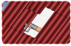
2. Fasten top screw of the roof hook to fix rails.
