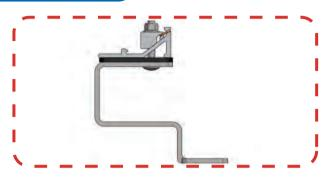
1. Fasten the bottom screw, fix hook to the wood beam.
